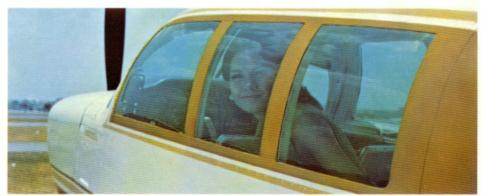
PANORAMIC VIEW . . . six big, wide-view windows in the EXECUTIVE and STATESMAN models give pilot and passengers excellent visibility. One-piece windshield presents a low drag frontal area. Trim-line center post is stainless steel for maximum strength and minimum compass deviation.
