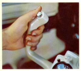
PC is standard equipment on all Mooney aircraft except the CADET. A PC release button is located at pilot's thumbtip in the ram's-horn control yoke. Press the button and Positive Control is disengaged; release the button and, unassisted, the aircraft returns to wings level attitude in a positive, coordinated maneuver.
